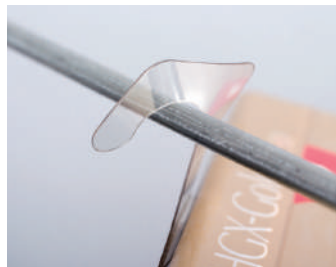
DEFLECTION: Hook unwinds and begins to fail due to overloading.
