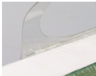
PEEL: Compromised adhesive bond due to overloading
