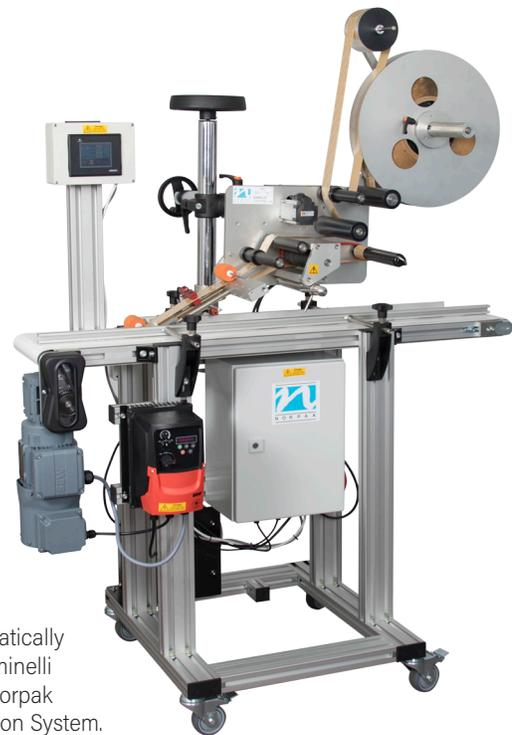
The R-J27 is automatically applied to the Creminelli package using a Norpak Hang Tab Application System.
