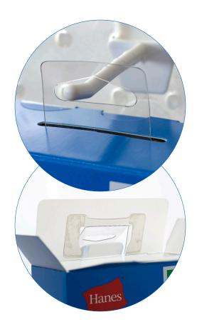
Do-It's R-5125 Hang Tab securely attaches to the inside of the Hanes product box. The hang hole portion of the clear 20 mil plastic hang tab fits neatly through the die cut slot at the top of the package. The result is a sturdy hanging package that sets Hanes apart from the competition and remains attractive in any retail environment.
